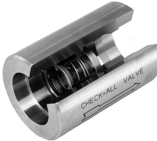
The **Universal Socket Weld (US)** check valve is a one piece body machined from bar stock with socket weld ends and is designed for a minimum pressure drop. It carries rugged, dependable Check-All® trim and there are a wide variety of seat materials and cracking pressures to choose from. The socket ends are machined to ASME/ANSI B16.11 dimensions. The US valve can also be used as a low pressure relief valve or vacuum breaker by using the desired spring settings.
