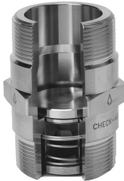
The **Connector (CN, CR)** valve is a check valve with a pipe nipple or connector housing. It is designed to be used in installations where a check valve with male pipe threads is required. The CN valve is adaptable for use as a low pressure relief valve or vacuum breaker by using the desired spring settings. Two valves used in combination make an excellent pressure vacuum vent. NPT threads are per ASME B1.20.1. Also available with ISO 7 "R" threads (CR).
